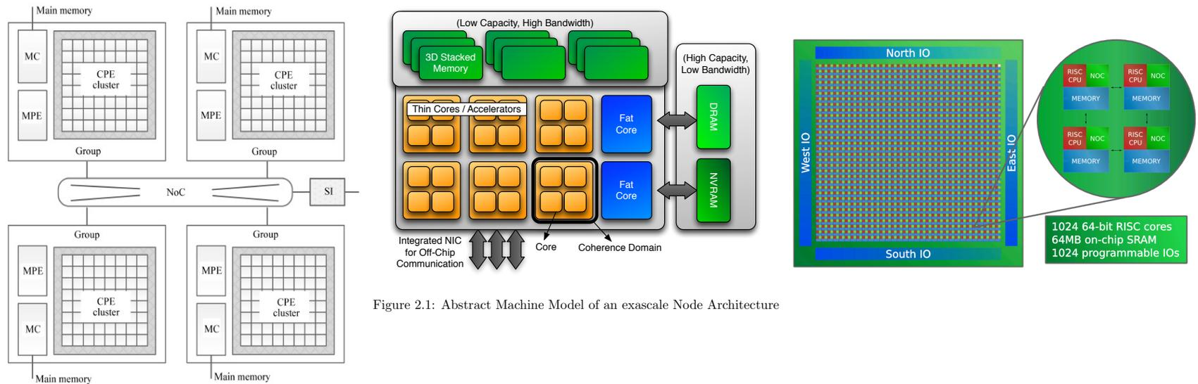
Figure 2.1: Abstract Machine Model of an exascale Node Architecture
