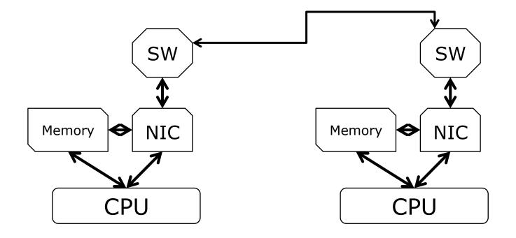
• Example path of data from one node to another: Using remote direct memory access
