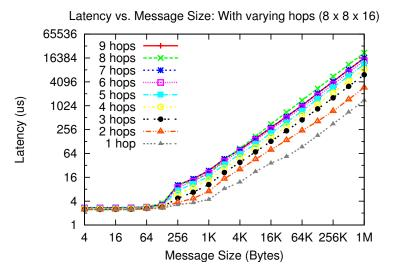
This example from IBM BG/P using messages between equidistant pairs; from "Quantifying Network Contention on Large Parallel Machines", Bhatele and Kale
