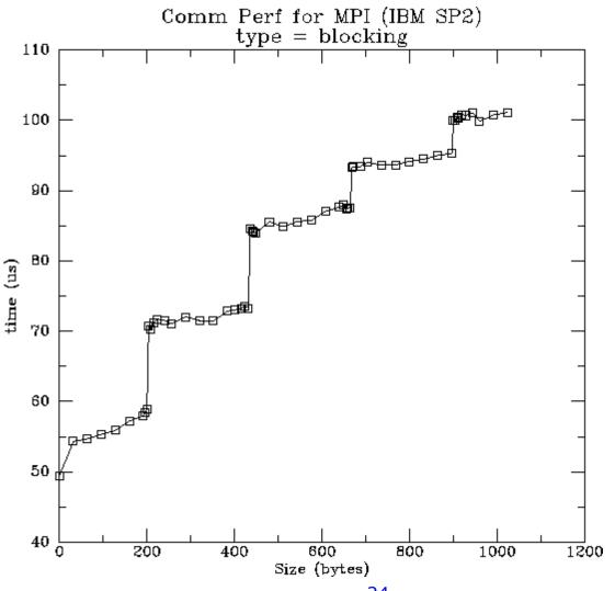
Packets contain 232 bytes of data. (first is 200 bytes, so MPI header is probably 32 bytes).
